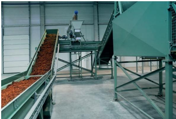
4. Peat raw materials and constituents are carefully dosed in controlled ratios onto the transportation belt.
