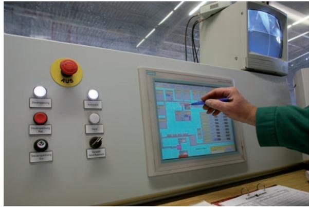
3. Computerised control of production in real time, each substrate has its specific recipe filed in the control computer
