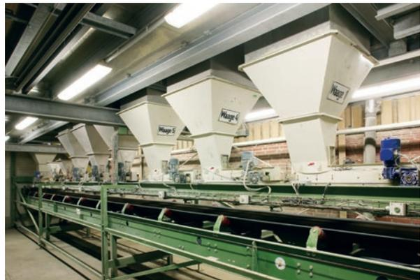
5. Addition of lime and fertiliser, weighing hoppers for exact dosing of fertilisers
